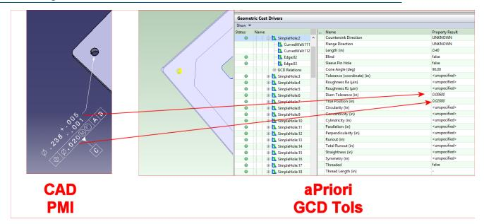
In this example, note that the "+.005/-.001" CAD PMI tolerance appears in aPriori as a total ".006" tolerance.
