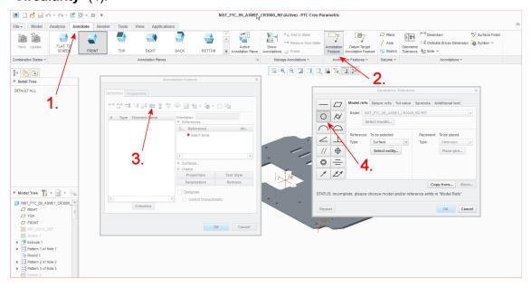
2 In the Geometric Tolerance dialog box, click Select entity (1), then click the surface to be associated with the tolerance (2). Then click Place gtol (3) and again click the associated surface (4).
