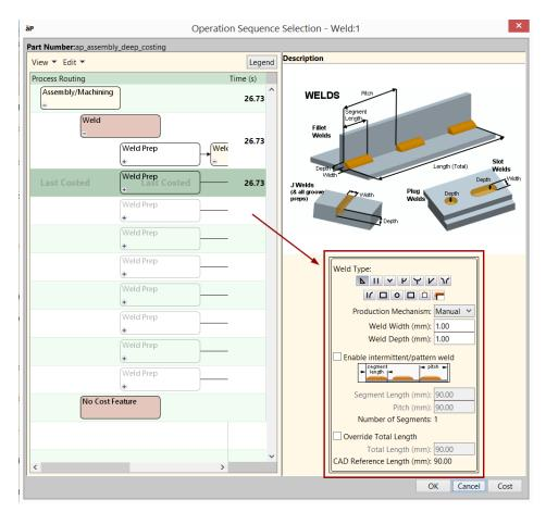
This dialog allows you to specify **Type**, **Width**, **Depth**, **Segment Length**, **Pitch**, and **Total Length**, as well the **Production Mechanism** for the weld (Manual or Robotic). aPriori computes the weld's **Volume**, **CSA** (cross-sectional area), and **Number of Segments** based on the other properties.
