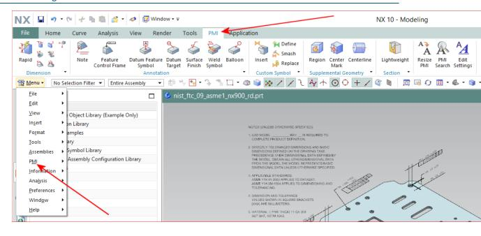
3 To specify and apply geometric tolerances to model features, click either the Feature Control Frame icon in the tool bar, or Menu > PMI > Feature Control Frame, then fill in the fields on the Feature Control Frame dialog.
