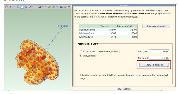
To modify the maximum and minimum thickness thresholds, click the **Manual Input** radio button and enter values into the **Max** and **Min** fields. Then click **Show Thickness** to display thickness violations in the Viewer using the modified thresholds.
