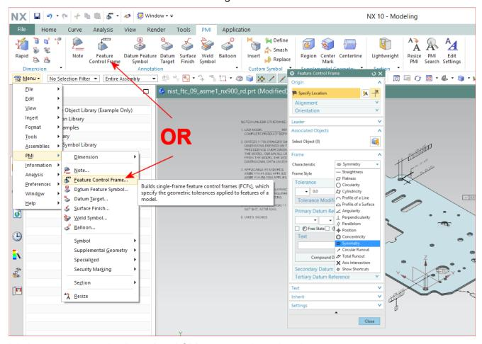
It is important to use the **Associated Objects** control to select the correct geometry reference (typically a surface or a hole) and associate it with the annotation you are creating. Note that aPriori does not read PMI associated on edges.
