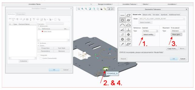
3 Select the dimension that was just added to the surface, and then click **Ok** in both the **Geometric Tolerance** dialog box and the **Annotation Feature** dialog box.
