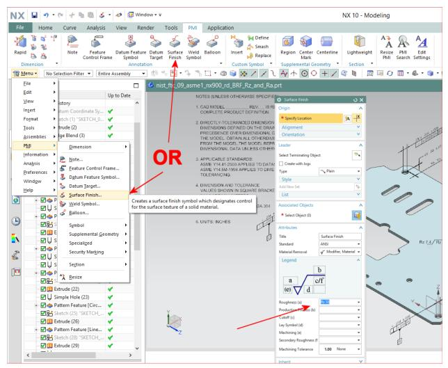
As mentioned with above for GD&T PMI, you must use the **Associated Objects** control to select the correct geometry reference and associate it with the roughness annotation you are creating.
